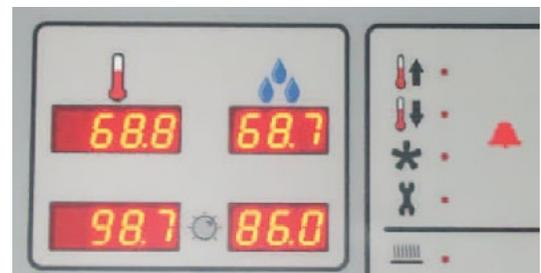
Large, high-contrast LED displays enable current conditions in the incubator or hatcher to be seen clearly at-a-glance.
